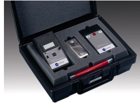
Periodic Verification System B48115PVS
